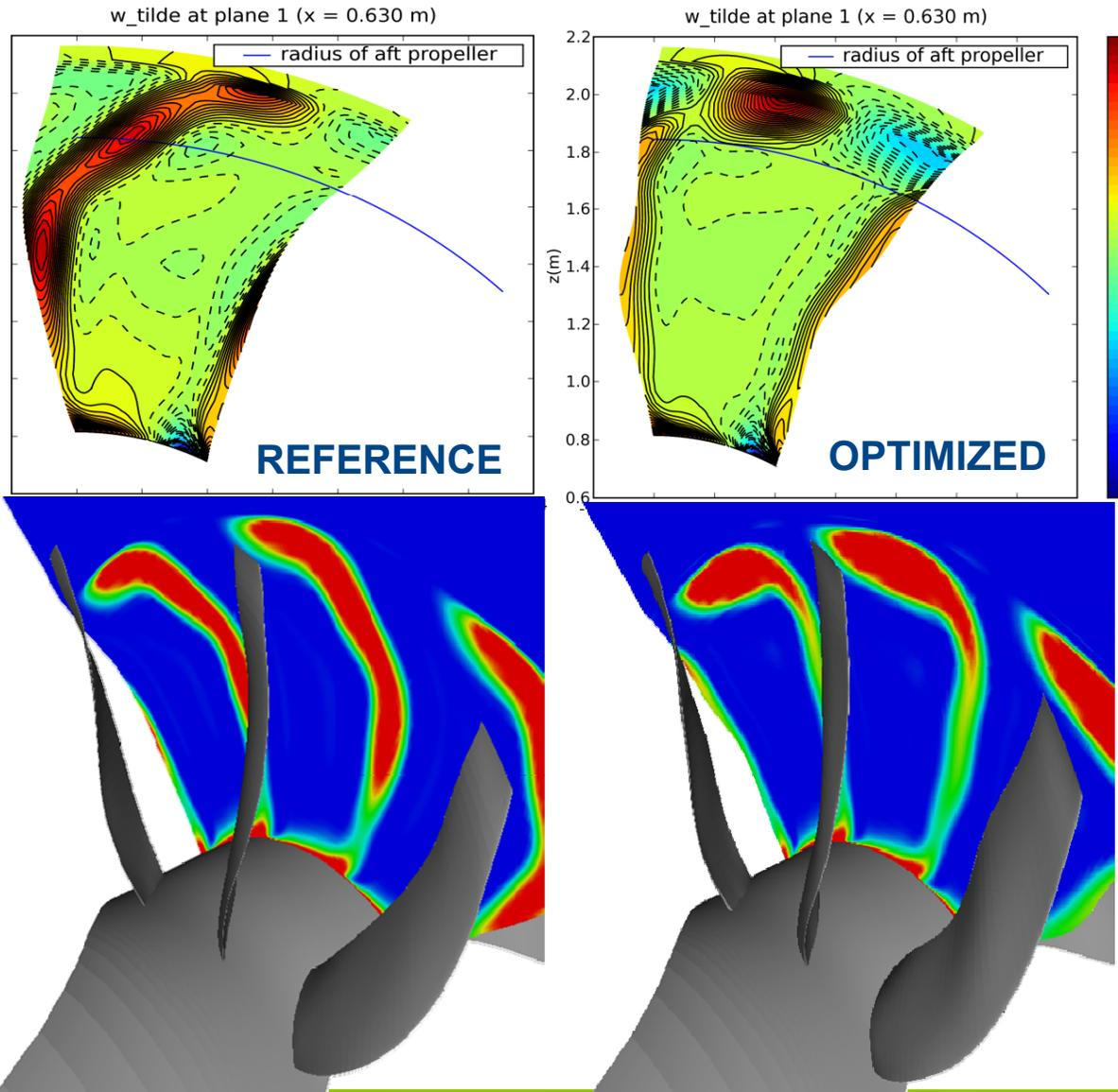
Acoustic criterion may be seen as “minimization of R1 wake, up to the height of R2”
